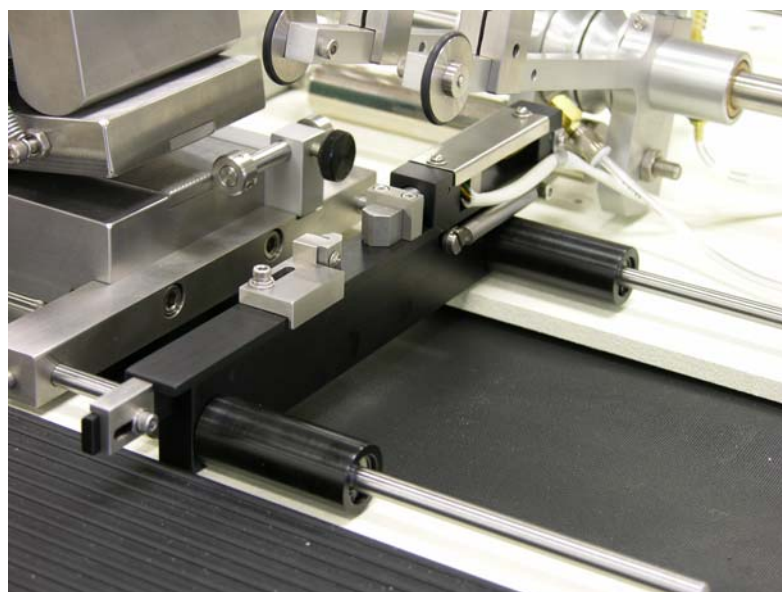
Fig 1. Model HMH-50-2 mounted to a 5,000 lbf horizontal tester
