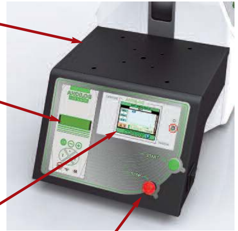
Separate control panel to setup the displacement of the test stand
