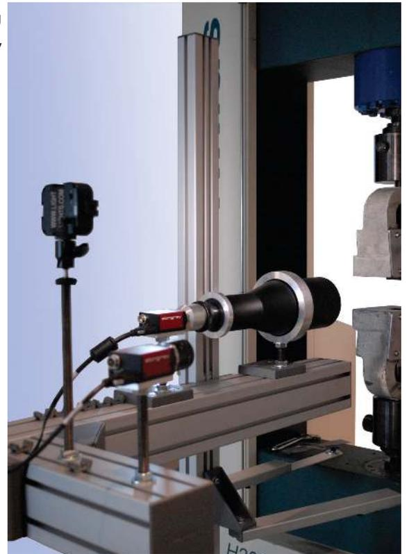
Dual camera setup, one camera with materials testing lens and the other camera with a general purpose lens; also showing mounting bracket and light source (if required).
