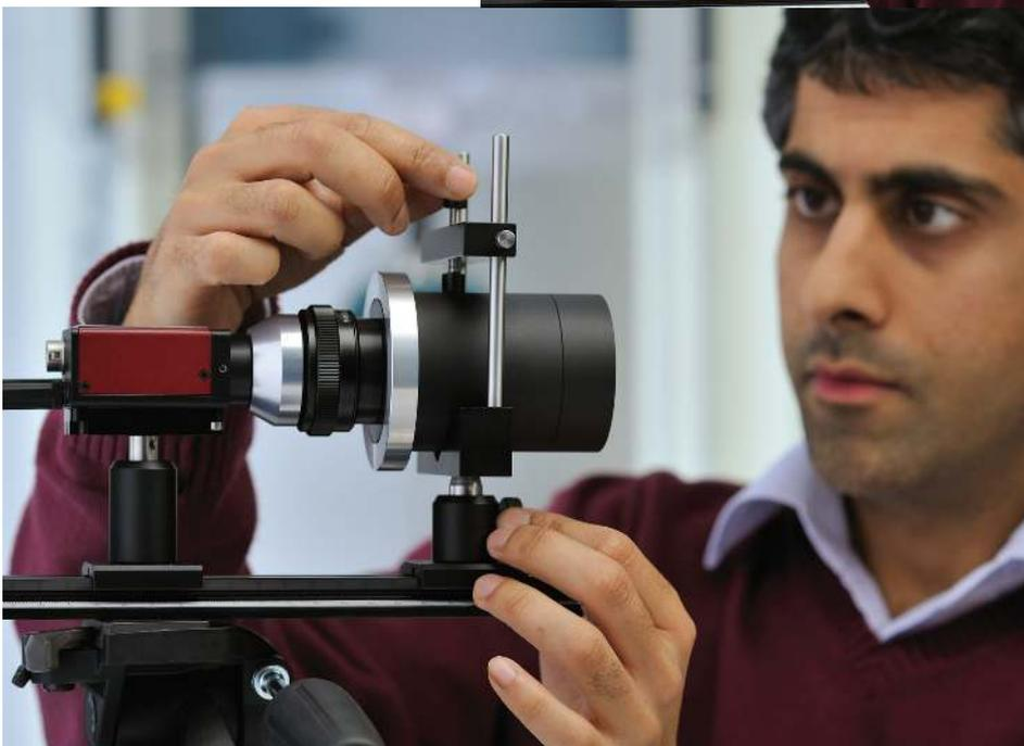
Video camera lens being switched to a general purpose lens to allow testing of more elastic materials.
