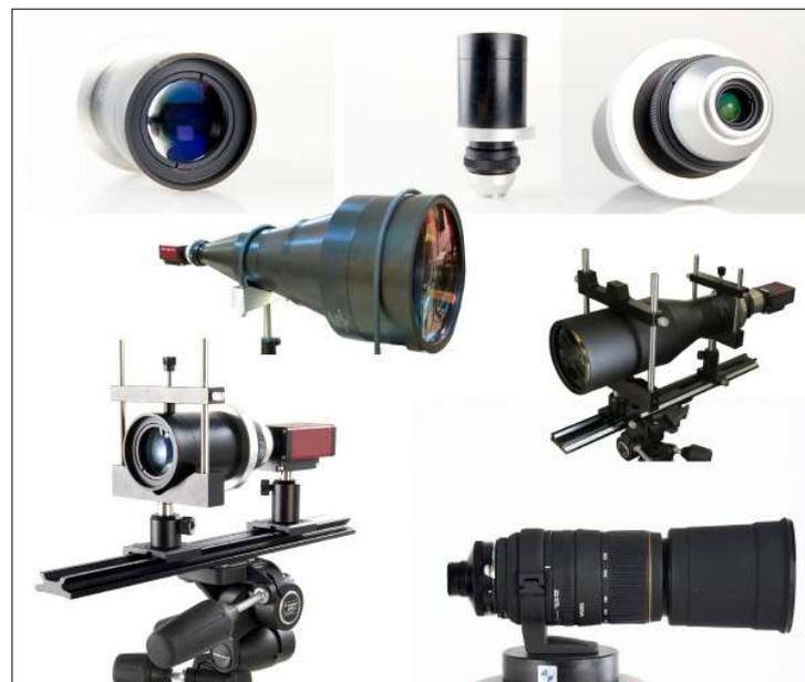
Selection of materials testing lenses, some shown with different translation stages that support the camera and lens and allow movement for focusing.
