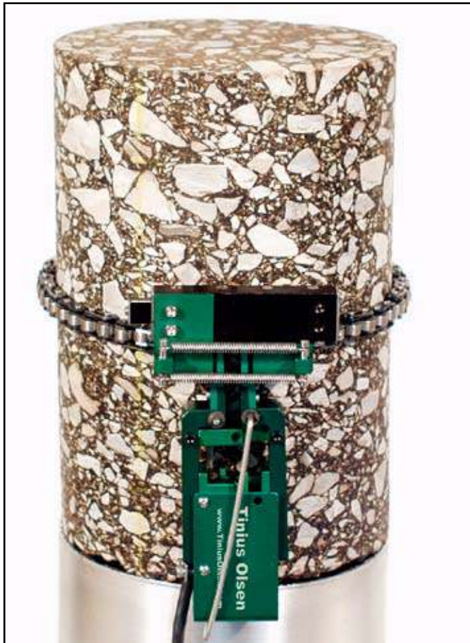
Figure 1. Model 3544 circumferential extensometer.
