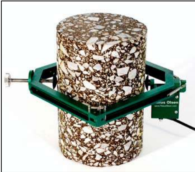
Figure 2. Model 3975 circumferential extensometer.
